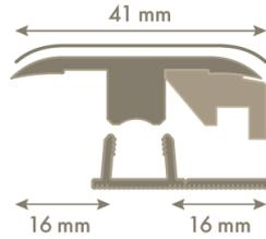
First saw the profile to the right length. Cut section B away with the knife to make an edge profile.
