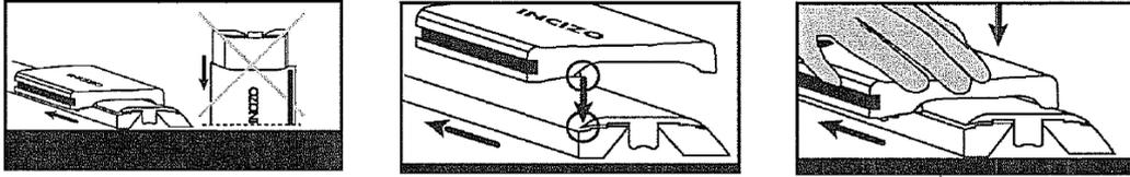
Always place the profile horizontally on a stable base when cutting.
