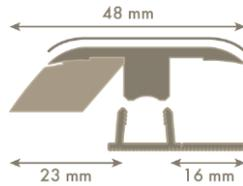
First saw the profile to the right length. Cut section A away with the knife to make an adapter profile.
