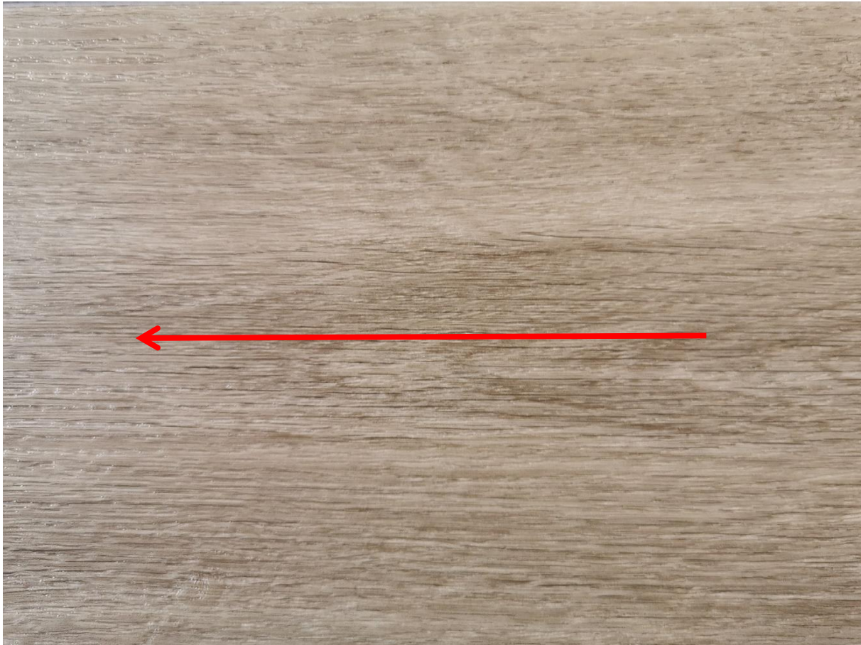
Figure 1: Vinyl plank - Titan Ridged 6 mm Arrow indicates direction of testing
