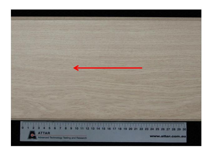
**Figure 1:** Quick-Step IM/IMU3105 Laminate White Varnished Oak Arrow indicates direction of testing
