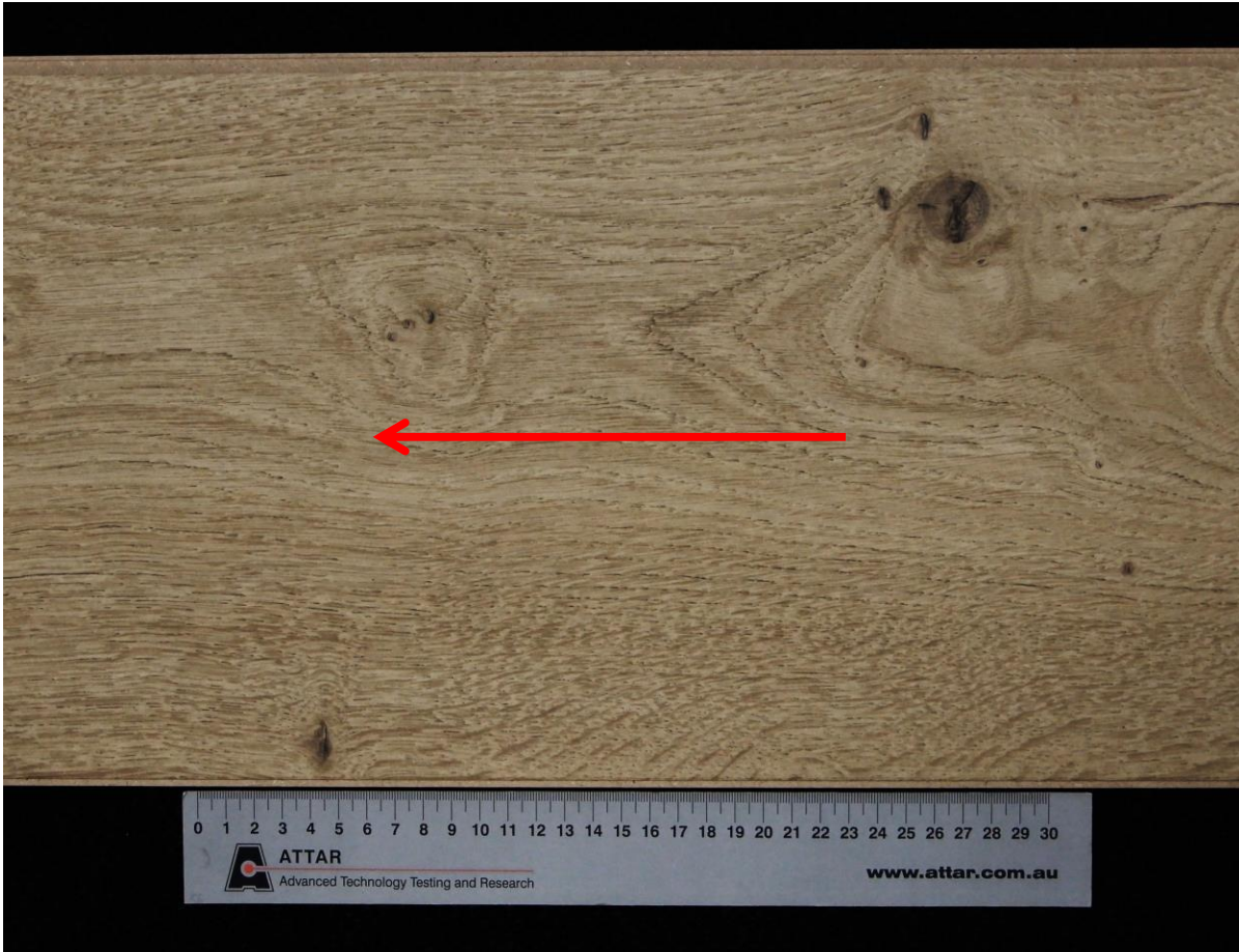
Figure 1: Pergo Odense Laminate 9.5mm Solstice/Glacier/Beaufort Oak Arrow indicates direction of testing
