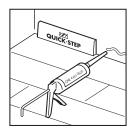
Fix skirting boards or scotia using quality construction adhesive and/or brads or small diameter nails. It is important to never attach or glue the skirting board or scotia trims to the floor. This method allows the floor to expand and contract under the profile. In places where profiles, skirting-boards or scotias cannot be placed (around steel door frames etc), Quick-Step hydrokit can be used to fill the expansion gap.
