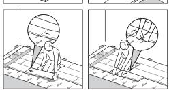
In places where it is too difficult to install the Uniclic® planks with the tapping block (e.g. against the wall), you can tap them together using the pulling iron and a hammer.
