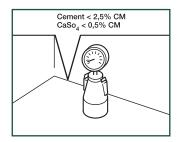
The moisture content of the subfloor must be less than 2,5%CM / 75%RH (cement screed) or less than 0,5%CM / 50%RH (anhydrite screed - subfloor). In the case of floor heating, results must be respectively 1,5%CM / 60%RH and 0,3%CM / 40%RH. Always measure, record and keep your moisture content results.
