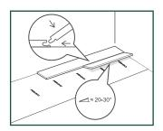
In order to make the start of the installation easier, assemble the first 3 rows away from the wall, so you can sit on the planks during the assembly. Then slide the first 3 rows at the wanted position close to the wall with distance spacers in place.
