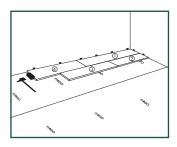
If method A is not possible (at hard to reach places by example), you can use method B (tapping): With Uniclic® you can also join the panels, by tapping the planks into each other, eliminating the need to lift them. This method requires the use of the special Uniclic® tapping block.
