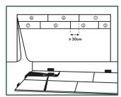
In places where it is too difficult to install the Unilic® planks with the tapping block (e.g. against the wall), you can pull them together using the pull-bar and a hammer.
