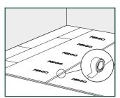
We strongly recommend to use the special PERGO rigid vinyl underlays. They have a noise-reducing and leveling function. The smooth top surface of the underlay makes installing the PERGO rigid vinyl panels easier and allows floor shrinkage and expansion afterwards.
