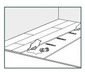
It is recommended to make additional checks of the straightness, in order to confirm the straightness during the installation. Remember to use the distance spacers for the expansion gap of 8mm (0,315 inch) along the perimeter.
