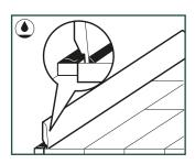
Install the skirting-board with Pergo Multiglue against the wall. When choosing the colour matched skirting or scotia, use the respective hydrostrips to avoid ingress of water and to obtain the look of a cleanly kitted finish. The waterproof paintable skirting can be used without a hydrostrip.
