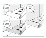
It is recommended to install the first strip of underlay, parallel to the long side of the PERGO rigid vinyl floor and gradually add strips of underlay as you progress the floor installation. When installing the next line of underlay, it is recommended to connect the underlays using a thin adhesive tape to avoid overlapping.
