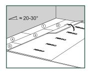
After the installation of each plank and before continuing with the next plank, check each short and long side joint to make sure there are no height differences and no openings.
