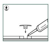
Fix the Incizo base profile to the subfloor with Pergo Multiglue. Apply the flexible Sealant on the PE foam that is in the expansion joint.
