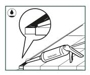
Sealing the perimeter expansion joints combines a compressible PE foam and the flexible and waterproof Pergo Sealant. Place the PE foam in the expansion joints with the help of the self-adhesive backing and apply the flexible Pergo Sealant under slight angle towards the Pergo floor. Make sure that the Pergo Sealant covers about 1 to 2 mm of the wall, the whole foamstrip and 1 to 2 mm of the floor.
