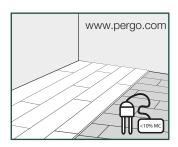
In case of installation on a wooden subfloor, please remove any existing floor covering first. No signs of mold and/or insect infestations should be present. If there is moist in the woodbased subfloor or there is no proper moisture barrier below the woodbased subfloor it has to be removed first. Reason is that the wood wil rot after time because the moist is blocked by the new flooring and its underlay.
