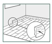
Inspect the final surface of the installed floor. Install PERGO vinyl skirtings against the wall but never attach the skirting to the floor itself. This method allows the floor to expand and/or contract under the skirting-board.
