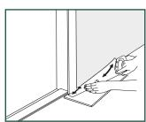
Do not fill or cover the expansion joints with silicone or other kit. If you would like to finish your floor fully waterproof, read the instructions below "3. FINISHING IN ROOMS LIKE BATHROOMS, KITCHENS, LAUNDRY ROOMS AND ENTRANCE AREAS" before installing the skirtings.
