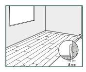
Room temperature varies continuously, so it is vital that the floor is able to expand and contract. For this reason, make sure you leave an expansion gap of 8 mm on all sides of the floor, around pipes, thresholds and under door frames. Expansion gaps can be finished by means of a skirting that is attached to the walls or with an expansion profile. In most cases you don't need an expansion profile between different rooms. However, the use of an expansion profile is mandatory when
