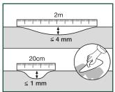
Cement joints between tiles or other gaps of more than 2mm (0,08inch) in depth and 5mm (0,2inch) in width should be levelled.
