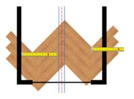
A square board of 20mm 580mm x 580mm x 580mm MDF, particle board or ply can be temporally fastened to the sub-floor to aid in aligning the herringbone correctly and also as an immovable object to work off. Having a firm vertical surface is useful for initially getting setup and helps prevent the panels from moving around when tapping them together.
