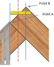
In instances where the entrance of the dwelling is the main priority of focus the herringbone pattern should be aligned to the centre line of the hallway.
