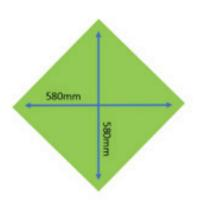
Boards should have the tongue facing out from the square board. Board 1 should be installed first and then followed by board 2 and so on,
