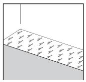
Underlay is essential for all laminate installations. The specially designed Quick-Step underlays feature damp proof, insulating and noise reducing properties as well as the ability to take up minor subfloor variations. The smooth top surface makes
