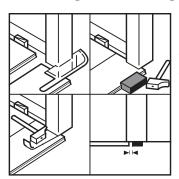
During the installation, an expansion gap will be left at the entire perimeter of the floor and where the flooring meets vertical finishes (skirting boards, walls, kitchen cabinets & kickboards, pipes etc). This gap will need to be covered after the installation has been
