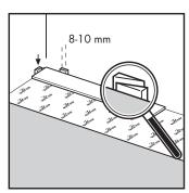
Roll out your Quick-Step Underlay one roll at a time in the same direction as the planned direction of the laminate floor boards. As subsequent rolls are installed, ensure the joins are taped using the underlays' integrated peel and stick tape. Any holes, tears or joins in underlay should be taped well using a vapour-tight tape.
