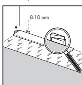
Roll out your Quick-Step Underlay one roll at a time in the same direction as the planned direction of the laminate floor boards. As subsequent rolls are installed, ensure the joins are taped using the underlays' integrated peel and stick tape. Any holes, tears or joins in underlay should be taped well using a vapour-tight tape.
