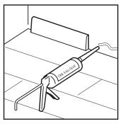
Fix skirting boards or scotia using quality construction adhesive and/or brads or small diameter nails. It is important to never attach or glue the skirting board or scotia trims to the floor. This method allows the floor to expand and contract under the profile.
