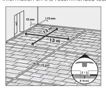
In general, the minimum perimeter gap is 10mm, however larger floors, or areas of high humidity may require larger perimeter gaps. Always use expansion joints to prevent runs exceeding 13 lineal metres in any direction.
