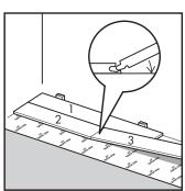
Continue now install the first board in the second row, ensuring that the end (or short) joins of any consecutive rows are at least 300mm apart to create a random staggered appearance and reduce wastage. Continue to install the boards as shown in the pictograms below and remembering to maintain the expansion gap using the spacers. After the first few rows are installed, use the offcut from the last row installed to start the next row.
