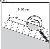
Roll out your Quick-Step Underlay one row at a time. As subsequent rows are installed, ensure the joins are taped using the underlays' integrated peel and stick tape. Any holes, tears or joins in underlay should be taped well using a vapour-tight tape.
