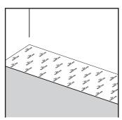
Underlay is essential for all laminate installations. The specially designed Quick-Step underlays have a damp-proof, insulating, noise-reducing and slight leveling function. The smooth top surface makes installing the laminate panels easier and allows the floors'
