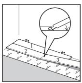
Continue now installing the first board in the second row, ensuring that the end (or short) joins of any consecutive rows are at least 300mm apart to create a random staggered appearance and reduce wastage. Continue to install the boards as shown in the pictograms below and remembering to maintain the expansion gap using the spacers. After the first few rows are installed, use the offcut from the last row installed to start the next row.
