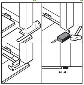
During the installation, an expansion gap will be left at the entire perimeter of the floor and where the flooring meets vertical finishes (skirting boards, walls, kitchen cabinets & kickboards, pipes etc). This gap will need to be covered after the installation
