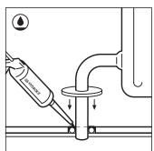
We recommend the sealing of the floor perimeter in bathrooms, laundries or other areas prone to have excessive amounts of water on the floor. This is to prevent water flowing in and under the floor at the perimeter. Sealing the perimeter expansion joints combines a compressible PE foam with diameter 8 to 10mm and the flexible and waterproof Quick-Step® HydroKit. Push the PE foam in the expansion joints and apply the flexible Quick-Step® HydroKit.
